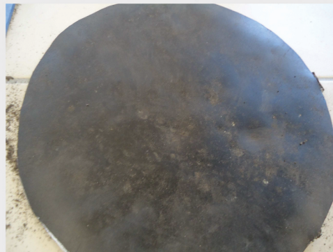
Lower surface of the test specimen MARISEAL 600
